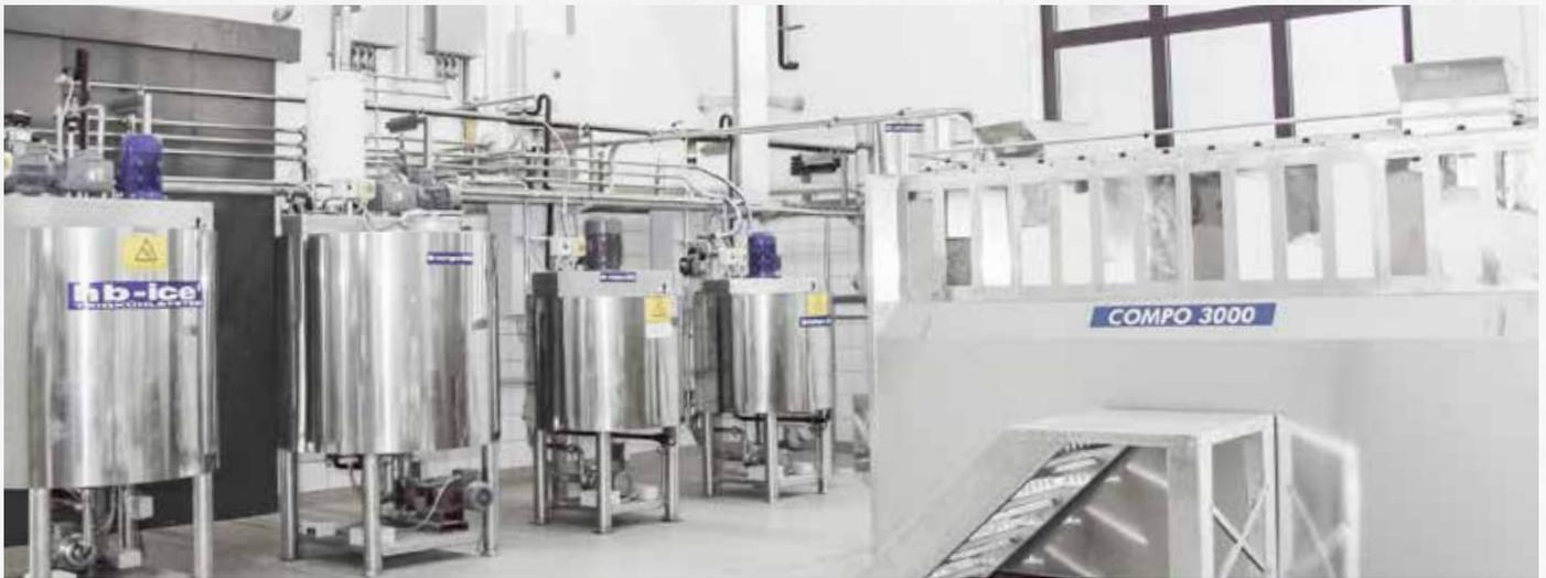
In the storage room of the Franziskaner bakery, the machines (from left to right) have been set up for the dough cooling system hb-ice®, for sour- and pre-doughs as well as the two small component containers Compo 3000 (behind one another).
