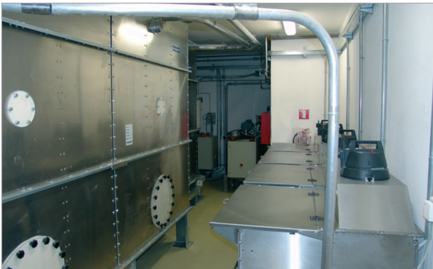
4 indoor silos, aluminium, rectangular, 4 dumping stations as daily silos
