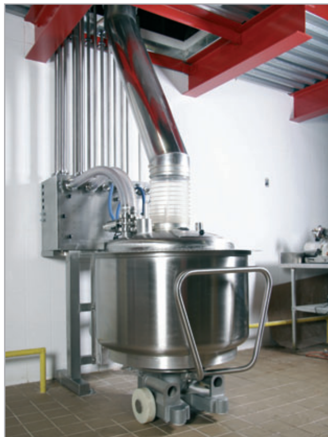
dust exhaustion hood with liquid dosing
